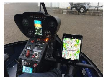
Make sure that the tablet is securely mounted. It must be mounted so it can be used without risk of interfering with other equipment and so that it will stay in place even in severe turbulence. Make sure that cables are not lying loose so they can interfere with the controls of the aircraft or any other equipment. With the new EASA rules on EFBs these recommendations are now explicit requirements!
