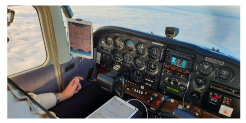
The following pictures are from a Cessna 172 where two ipads are used. One is mounted on a knee-board and the other with a RAM suction cup mount. The charging cable for the latter is a quality cable sufficiently long that in can follow the curve of the dashboard all the way around so it does not interfere with any controls or handles.
