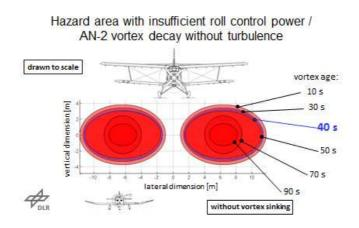
The graph of the hazard area of the wake vortex clearly shows that **in calm weather** the dimensions of the hazard area can still be so distinct approximately 1 - 1.5 minutes after the tip vortex generation that it poses a serious threat to aircraft such as a DR 400. Initially, the respective dimensions are approximately 11 m in width and approximately 6 m in height. Around the core diameter of approxi-
