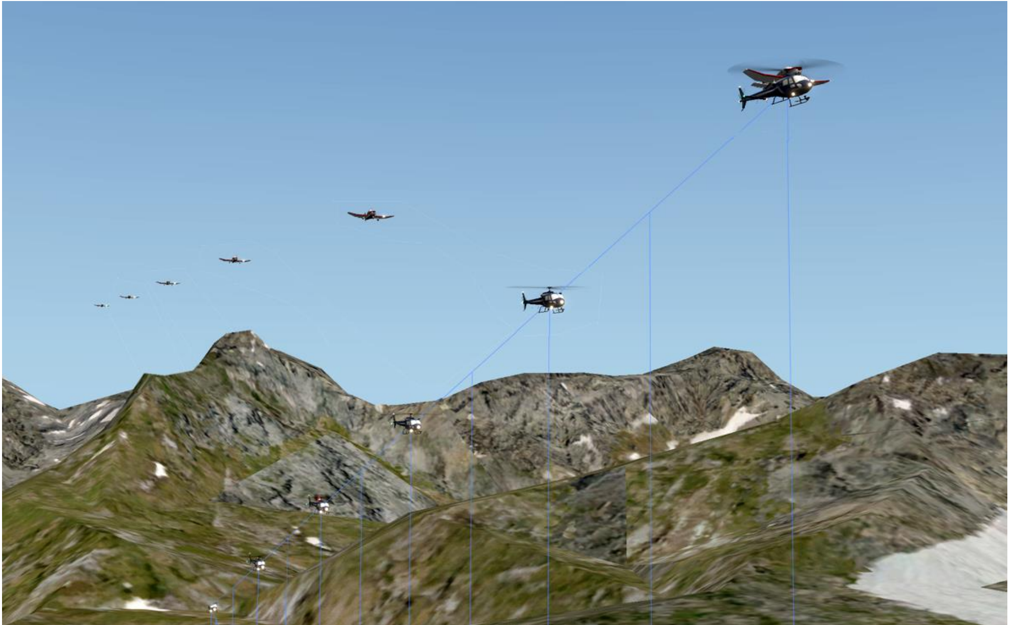
Figure 19: ANSV reconstruction of the trajectories of the two aircraft from ten seconds before the collision (from ANSV animation; the silhouette of a similar aircraft has been used to simulate the F-PMGV).
