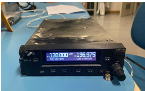
Photo 39: Garmin GTR 225A radio, recovered from the I-EDIC wreckage, powered in the ANSV laboratories.
