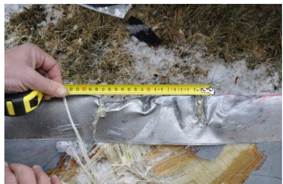
Photo 14: main rotor blade deformations due to impact against metallic parts.
