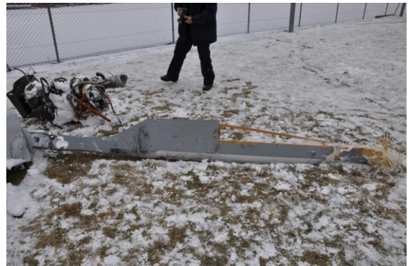
Photo 12: main rotor blade with outer section missing.
