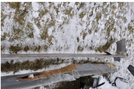
Photo 13: signs of red paint on main rotor blade.
