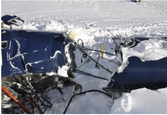
Photo 10: I-EDIC, tail beam disconnected from the fuselage.
