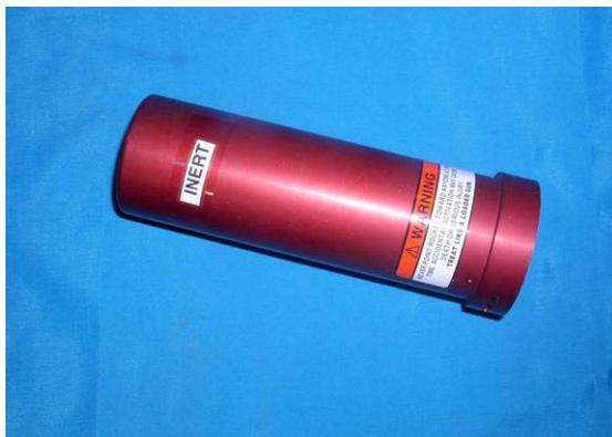
This is a close up of the **BRS 900** rocket motor, common to both Cessna and Cirrus installations. It produces roughly 225 pounds of thrust over a 1.2 second burn time and must be respected. It burns solid propellant derived from military formulations and is very resistant to accidental initiation.
