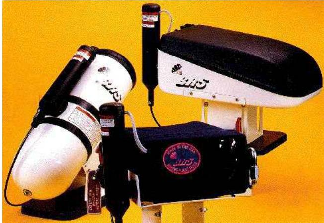
Used as intended, these BRS-brand emergency parachute systems have saved over 175 lives. More correctly stated - they save lives if used. However, the pilot must elect to deploy the system, completely different than, say, an airbag which deploys automatically when certain conditions develop. Because the pilot (or his passenger) must pull the activating handle, sometimes the units are not used.
