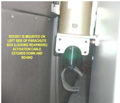
baggage area, as viewed from the front seats. The rocket is on the left of the parachute canister; the activation cable runs down to the floorboard, under a cover, then forward to the activation handle, located near the fuel selector.
