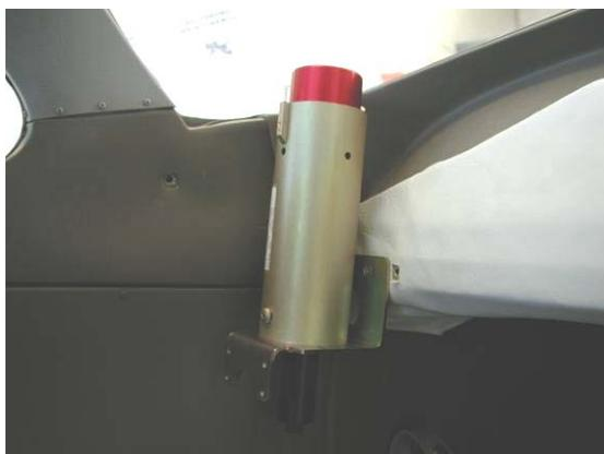
Here is another perspective of the **C172** rocket assembly with cover removed. It is just a few inches below the rear window, which it will readily break through when fired. Inside the launch tube resides the rocket motor, it's the red cylinder.
